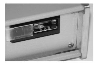
If it is not set for the proper voltage, remove the fuse and then grasp the card with a pair of pliers and remove it. Rotate horizontally through 180 degrees. Reinstall the card and the correct fuse.
